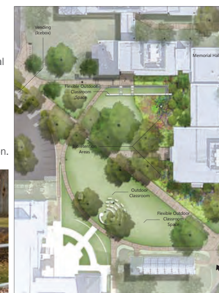
Detailed site plan for Memorial Hall landscape improvements and stormwater management (December 2014).
