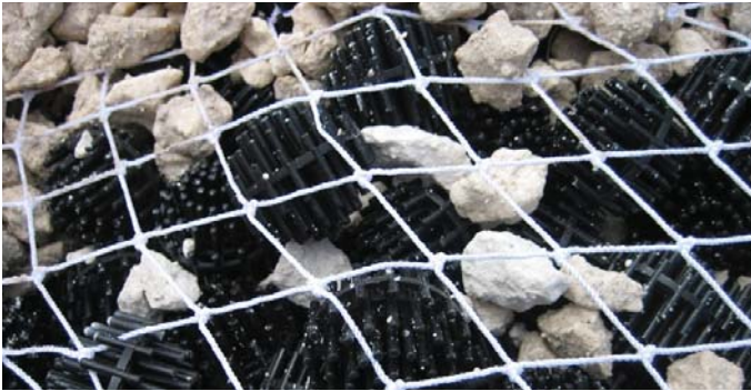
from top: Subsurface flow constructed wetland immediately after planting; Bioballs and gravel wetland treatment media
