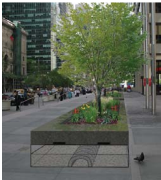
top: Simulation of stormwater swales integrated in parking lot design bottom: Simulation of stormwater planters with underground storage
