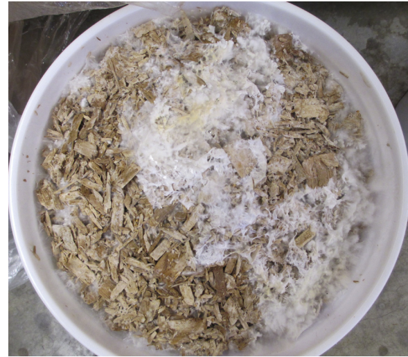
Fig. 2. Photograph of top of mycofilter with Stropharia rugoso-annulata on alder wood chips. Bucket was 0.26 m in diameter. Photo credit: Alicia Flatt.
