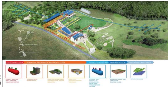
from top: Cross section of natural wastewater treatment & reuse system; Wastewater treatment wetlands flank the campus entrance; Campus-scale water treatment and reuse strategy
