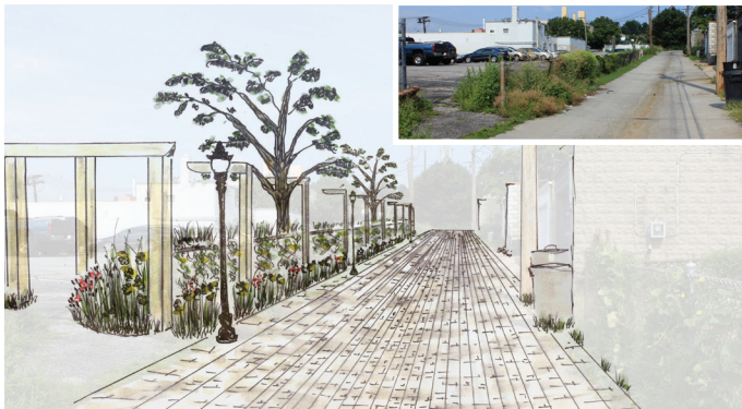
top: Photosimulation of stormwater tree pits and a rain garden on Belair Road with inset of initial conditions; bottom: Concept drawing of a green alley with permeable paving and new plantings behind Belair-Edison Family Health Center with inset of initial conditions
